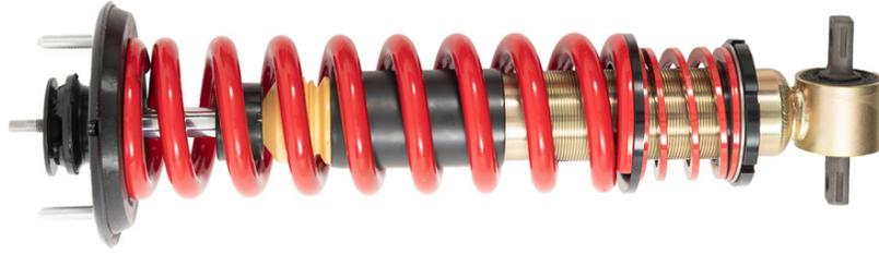
15. Confirm the vent disk is located on the strut, under the dust boot. If for any reason your vent disk is not present, please call our technical support staff before proceeding, as driving on the strut without it could cause the shock to fail.
